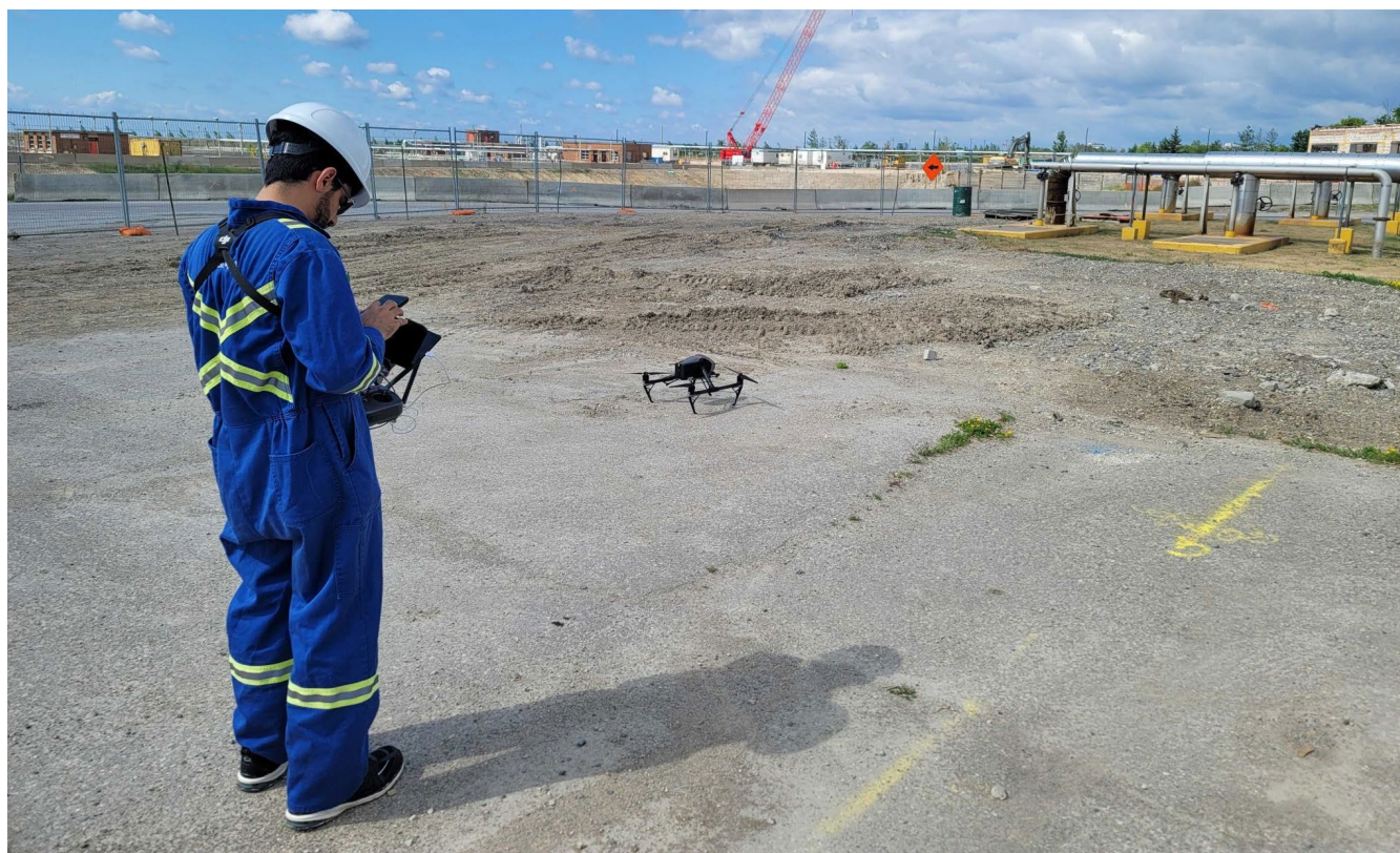
A Scentroid operator launches a DR2000-equipped drone at an active industrial site, maintaining a safe standoff distance from the sampling zone.
