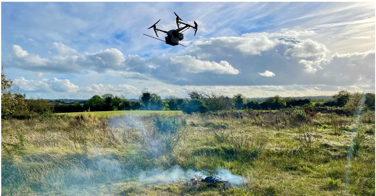
The DR2000's standoff sampling capability allows safe data collection near active combustion or flare sources and other hazardous plumes.
