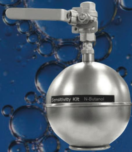
The Scentroid SK5 EN13725 Odor Panelist Sensitivity Kit is designed to provide accurate N-butanol mixtures of 4 to 40 ppm from a liquid N-butanol source. The N-butanol mixture can then be used to screen and odour panellist using the Scentroid SM100 or any other Scentroid olfactometer in accordance with standard EN13725.
