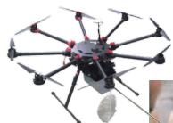
The DR1000 Flying Lab allows the operator to stay safely away from any hard to reach or potentially hazardous sources while acquiring the required air sample for laboratory analysis.
