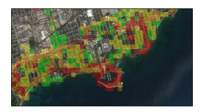
Urban Scanner comes with an intelligent cloud software which collects, analyzes, and visualizes the collected data. An advanced deep learning algorithm is used to generate geo-spatial predictions of urban pollution. This means that the system can provide pollution concentration values for locations that the Urban Scanner has not even sampled. The model can also be used to identify polluted zones and pinpoint the source of local pollution.
