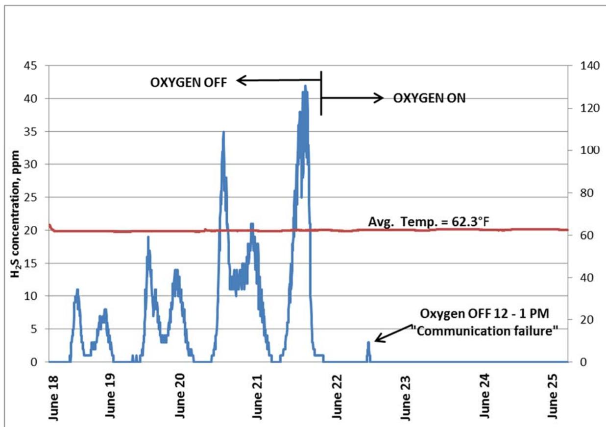
**FIGURE 3: H<sub>2</sub>S Concentrations at West Ave Pump Station 1mile downstream (SuperOxygenation System off and on)**
