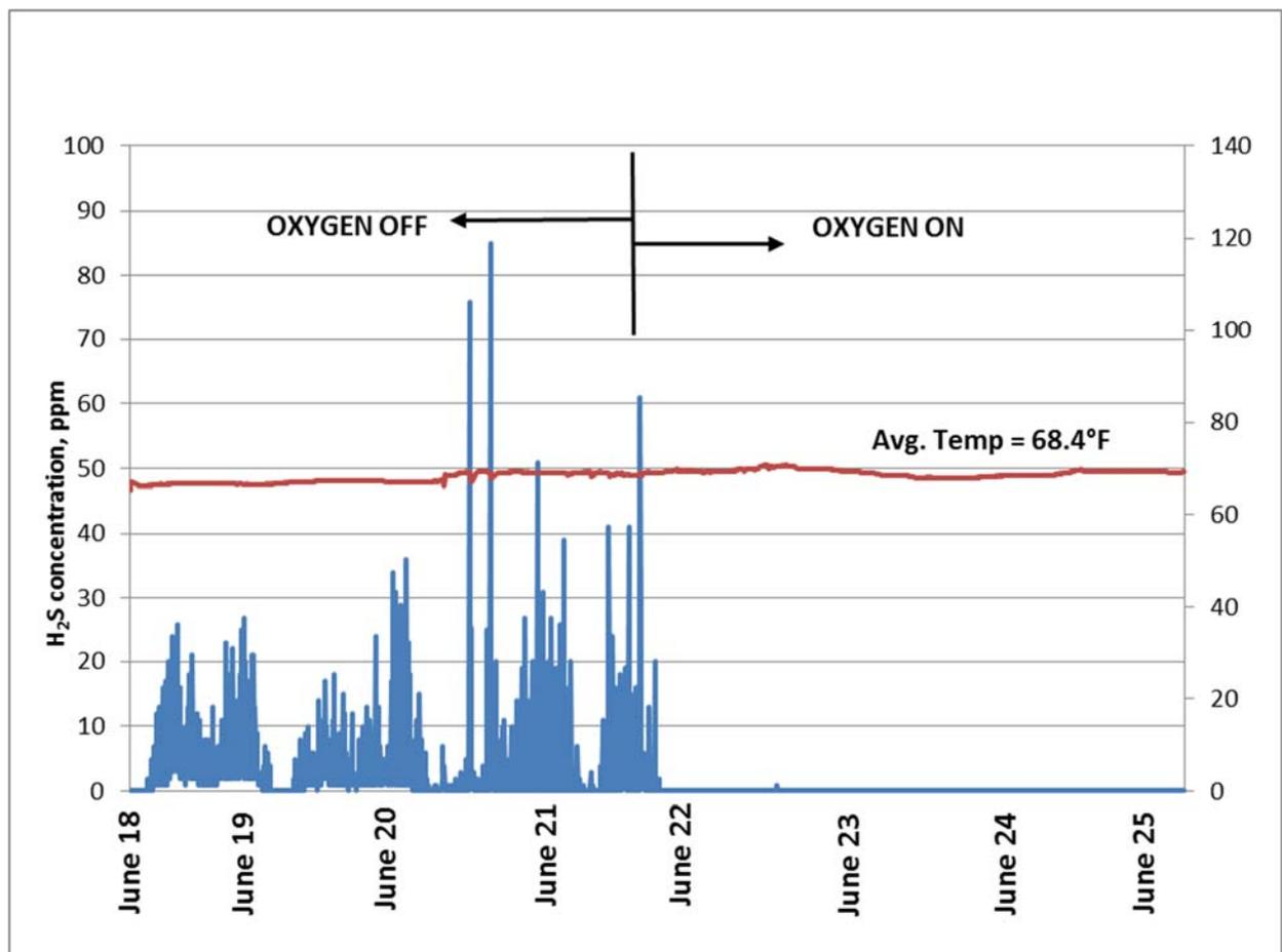
**FIGURE 2: H<sub>2</sub>S Concentrations at Gulf Pond Force Main Discharge (SuperOxygenation System off and on)**
