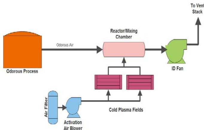
Fig 4: Injection odor treatment with Cold Plasma systems
