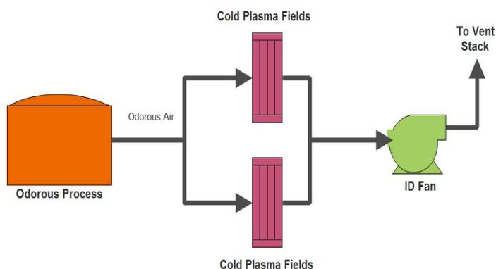
Fig 3: Flow through odor treatment with Cold Plasma systems
