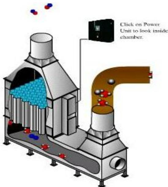
Fig 2: Typical corona, flow through system
