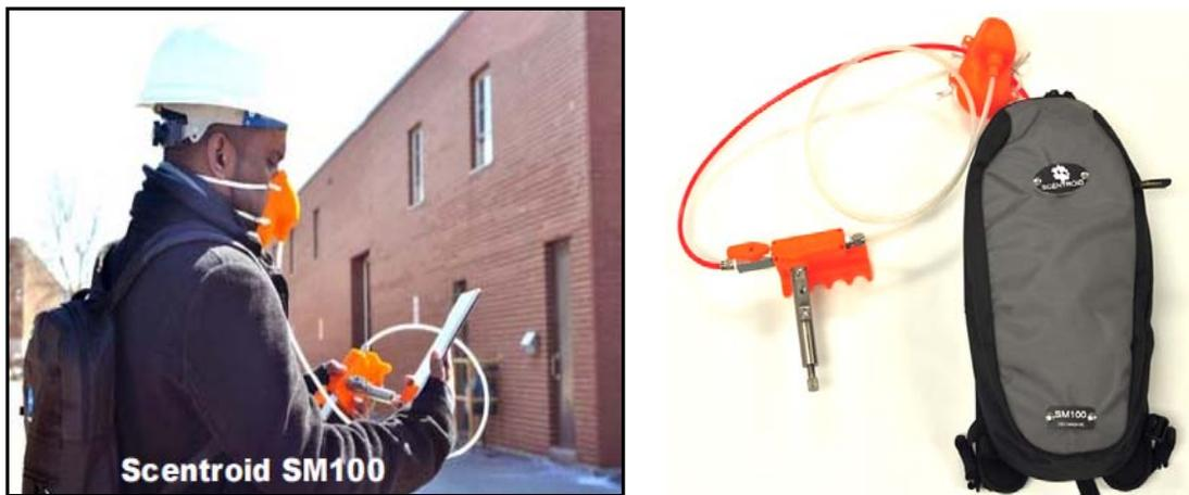
**Figure 2-1 Scentroid's SM100 Infield Olfactometer**
