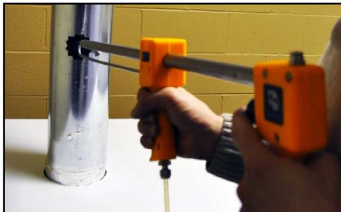
Figure 2-2 Scentroid's Stack Diluting Sampler
