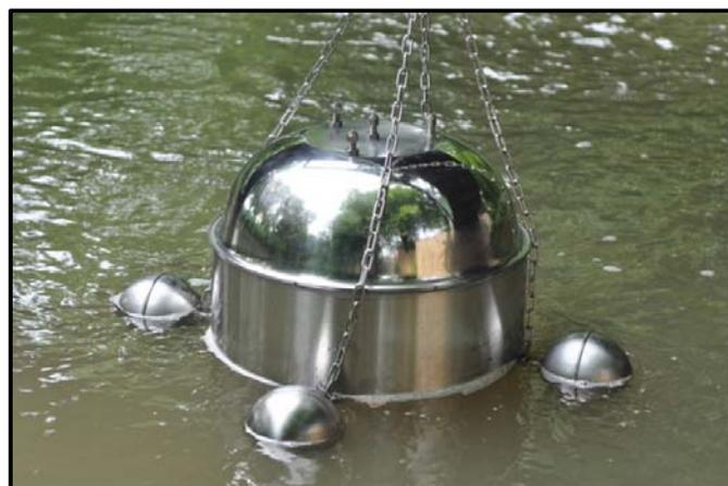
Figure 2-3 Scentroid's Dynamic Flux Chamber
